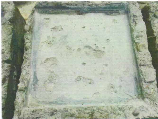
Photo 2: Left photo shows Sample 2 treated with ChemTec ONE solution and right photo shows Sample 2 untreated after 100 Freeze-Thaw cycles. Note severe deterioration of the non-treated sample and complete surface loss.
