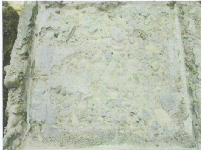
Photo 1: Left photo shows Sample 1 treated with ChemTec ONE solution and right photo shows Sample 1 untreated after 100 Freeze-Thaw cycles. Note severe deterioration of the untreated sample and nearly complete surface loss.
