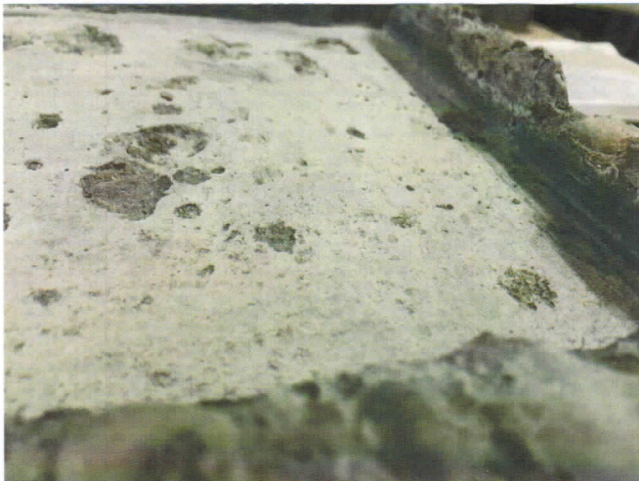
Photo 4: Close-up showing Sample 2 treated with ChemTec ONE solution (left photograph) and Sample 2 untreated (right photograph) after 100 Freeze-Thaw cycles. Note severe deterioration of non-treated sample and protruding coarse aggregate.
