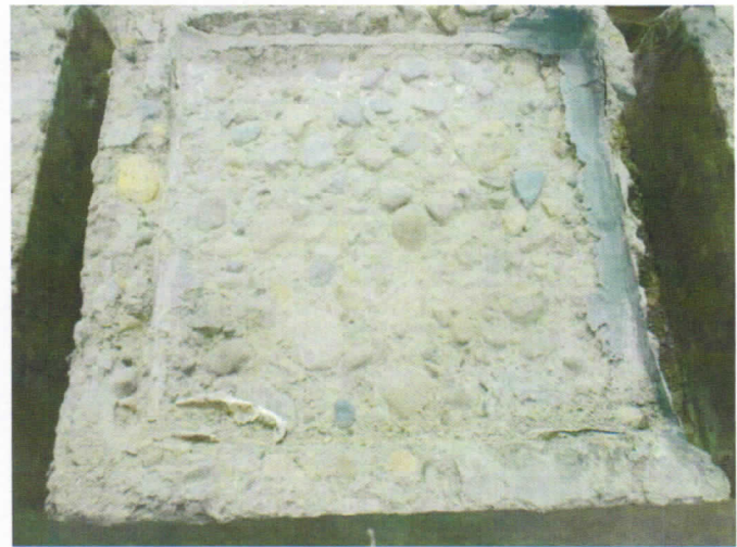
Photo 2: Left photo shows Sample 2 treated with ChemTec ONE solution and right photo shows Sample 2 untreated after 100 Freeze-Thaw cycles. Note severe deterioration of the non-treated sample and complete surface loss.
